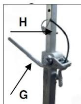
Position the drill mount. Position the clamping device as close as possible behind the column on the base of the mount. Fix the mount by turning the crank (G) clockwise.
