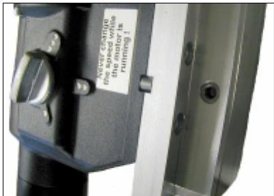
The drilling stand P-54190 comes with a mounting plate, a 10 mm fitting key and 4 hexagon hollow head plugs M8. The mounting plate is fixed on the tool with the fitting key so that the coupling on the mounting plate is on the same side as the gear change of the engine. The 4 plugs are then inserted and tightened.
